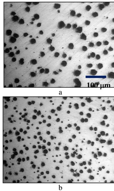
Fig. 6 Micrographs of the produced SGI with 40 mm thickness and 0.035 Mg%
