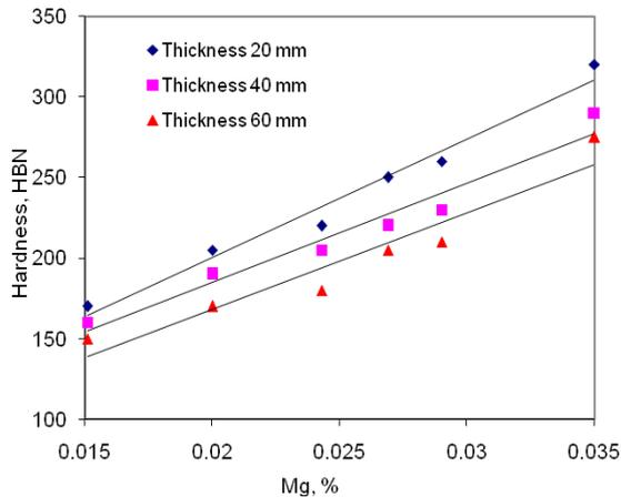
Fig 8 Effect of Mg contents on Hardness at different size
