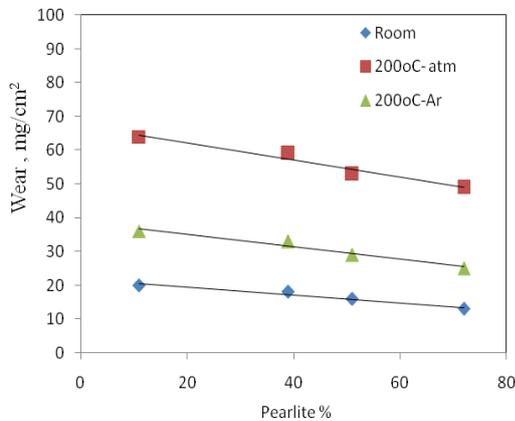
Fig. 11 Effect of Pearlite% on the wear amount of the produced SGI specimens at different elevated temperatures
