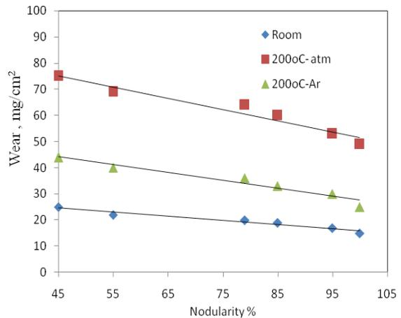
Fig. 10 Effect of nodularity% on the wear of the produced SGI specimens at different elevated temperatures and atmospheres.
