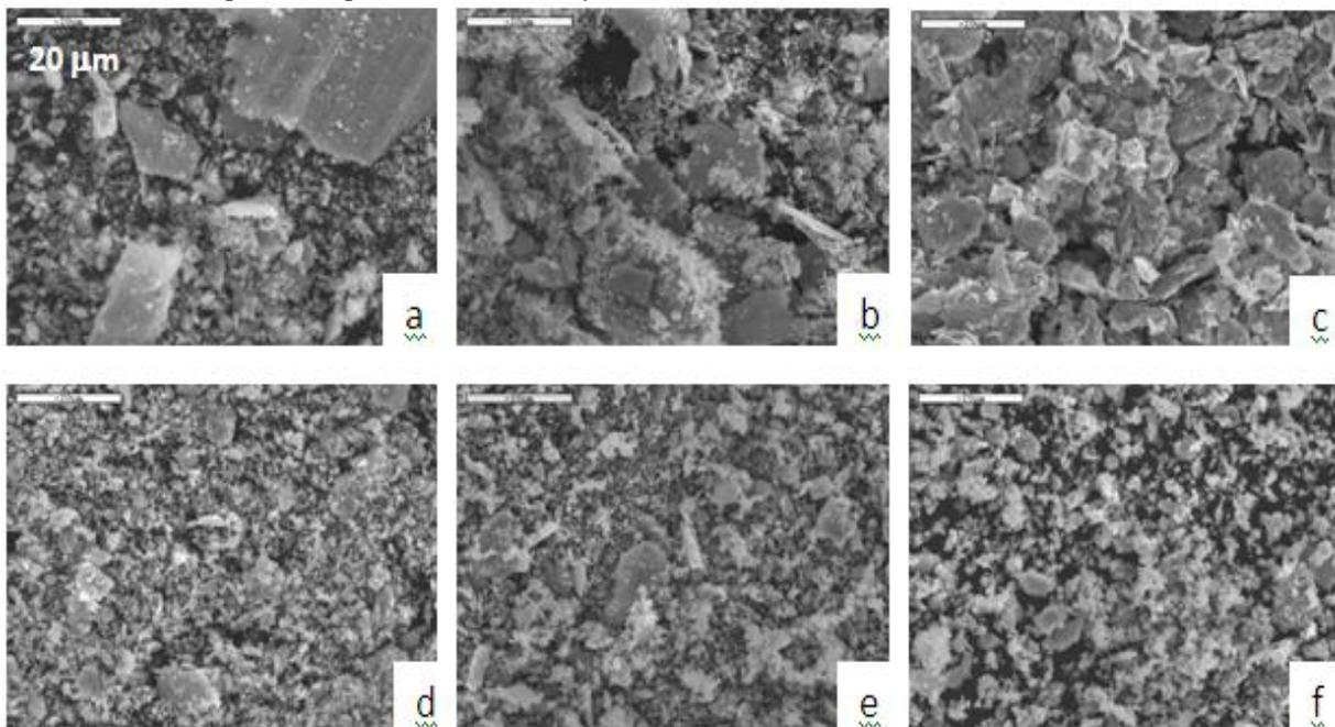
Fig. 12 SEM wear debris for SGI specimens at room temperature and different nodularity %, a) 45% b) 55% c) 78% d) 85% e) 95% and f) 100%.
