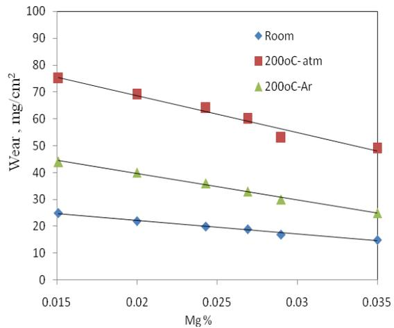
Fig. 9 Effect of Mg% on the wear of the produced SGI specimens at different elevated temperatures and atmospheres
