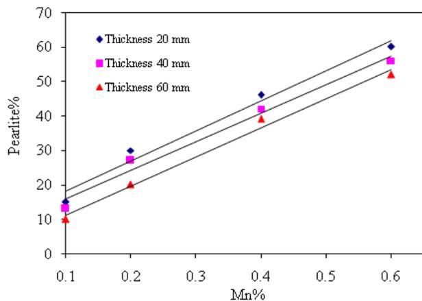
Fig. 4 Effect of Mn content on Pearlite in SGI at different thickness
