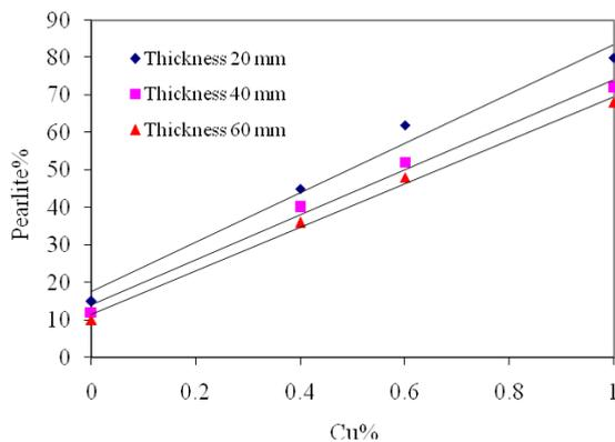
Fig.2. Effect of Cu content on the pearlite % in SGI at different thickness
