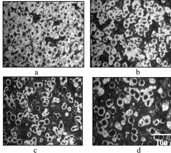
Fig. 3 Micrographs of the produced SGI at thickness 40 mm, 0.024% Mg and at different Cu contents
