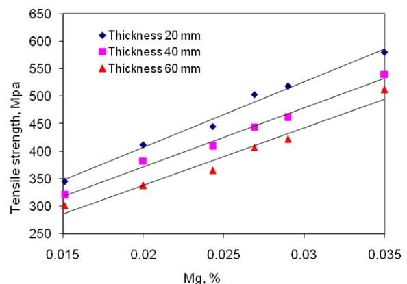
Fig 7 Effect of Mg content on tensile strength at different size
