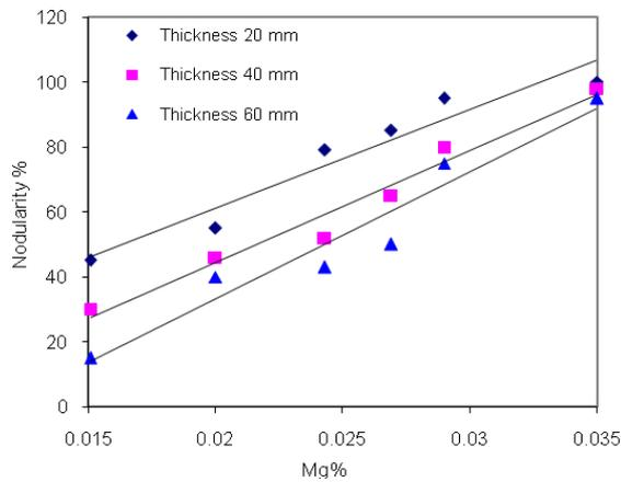
Fig. 2 Effect of Mg% contents on the nodularity% of the produced SGI specimens
