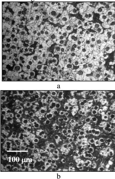
Fig. 5 Micrographs of the produced SGI at 40 mm thickness and 0.024Mg% with a) 0.1 Mn%, 13% pearlite b) 0.6 Mn%, 55% pearlite
