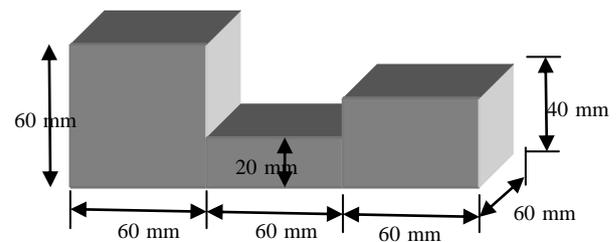
Fig.1. Schematic diagram for mold pattern and experimental setup to make different thickness
